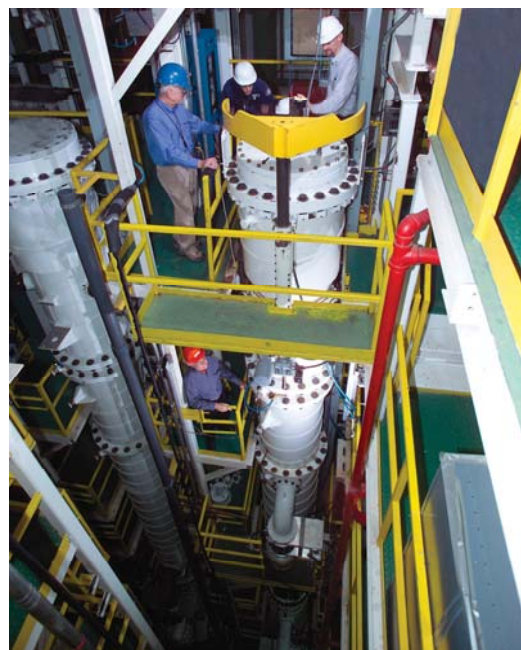
Fig. 3. Centrifuge test stand at the USEC R&D Center in Oak Ridge, Tennessee.
